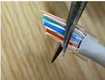
10 Push cable deep into the plug
